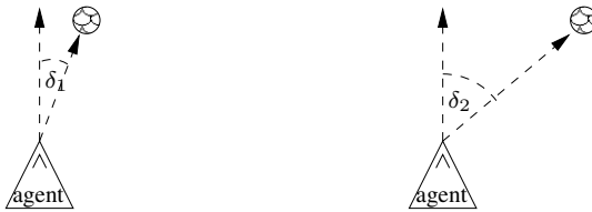
Fig. 5. Naïve ball interception: \delta_1 \leq \epsilon \rightarrow \text{run} ; \delta_2 \geq \epsilon \rightarrow \text{turn}
